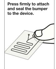
Continue applying bumpers to channel openings (inlets). Bumpers may also be attached to outlet openings if sample recovery is desired.
