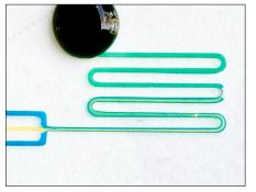
My prediction was partially correct, the dye did not mix at the crossing but one can see diffusion at the interface of the liquids that eventually results in the dye changing color by the end of the channel.
