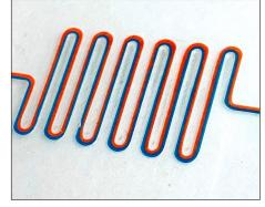
My prediction was correct, the dyes join at the crossing but do not mix because of laminar flow. They run together without obvious mixing to the end of the channel.
