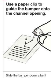
Slide the bumper down a bent paper clip onto the device. The perforation in the bumper should be centered directly over the channel opening.
